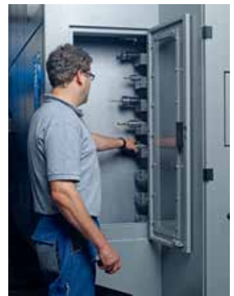
Setup during main time with the tool loading unit
